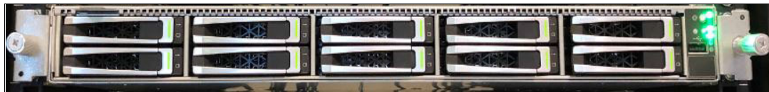
Figure 3-5 IBM Cloud Object Storage Accesser A10 front view
